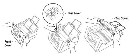
2 Remove the old print cartridge containing the used ribbon and dispose of it.
