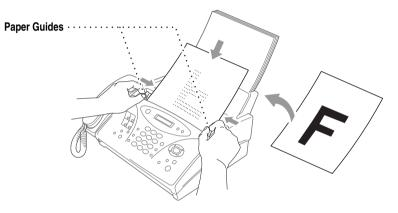
The automatic document feeder (ADF) can hold up to 10 pages, feeding each one individually through the fax machine. Use standard (17 lb–24 lb) paper when using the ADF; if you're using heavier paper, feed each sheet individually to prevent paper jams.
